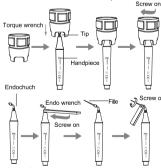
picture 2 Notes: The detachable handpiece is a hightech device which should be used carefully. Don't use too much torque force to screw the Screw the tips by torque wrench. In order to the vibration by touch the foot switch by accident, unscrew the scaling tips after each operation.
