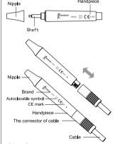
2.2 Installation of tips 2.2.1 Fix the tip to handpiece by torque
