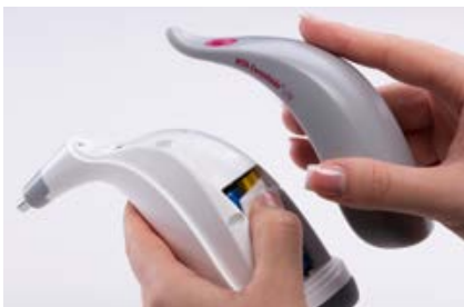
Figure 6 – Changing batteries: Replace top cover
