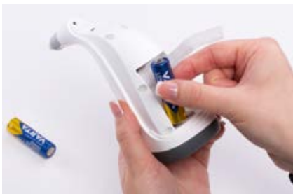
Figure 4 – Changing batteries: Remove battery on left
