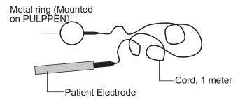
Place the PULPPEN tip on to the dried target tooth's surface. While maintaining contact with the tooth, touch the sensor button (10) with your index finger. The PULPPEN will emit electronic pulses through the tooth at a regularly increasing amplitude, as indicated by the pulsating red indicatorlight (LED).
