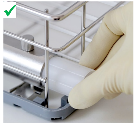
Fig. 4: Inserting the plastic central filter
