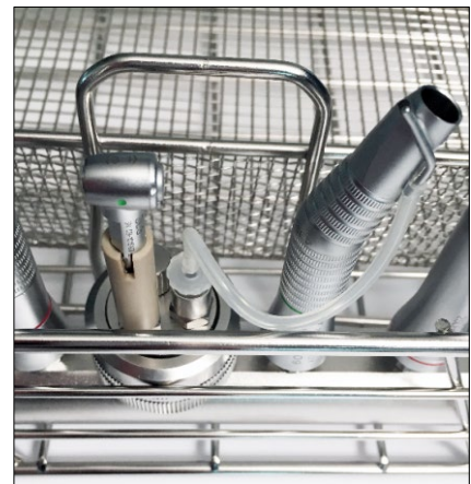
Fig. 34: The adapter is connected with the transmission instrument to be rinsed
