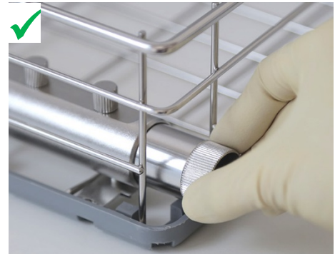
Fig. 3: Inserting the Cleanfinity Filter
