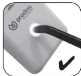
The lightguide (without protective cap) fits exactlyin the light measuring circle, point shows correct result.
