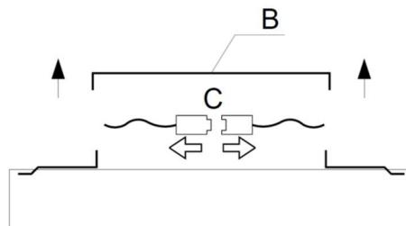
4. Lift the cover (B), disconnecting the connectors (C).
